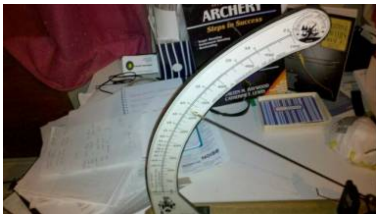
Fig. 2 - The arrow tests out at 42 pounds
