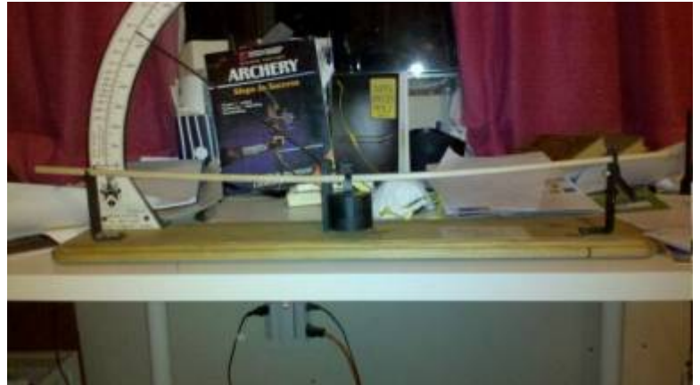
Fig. 1 - An arrow spine tester
